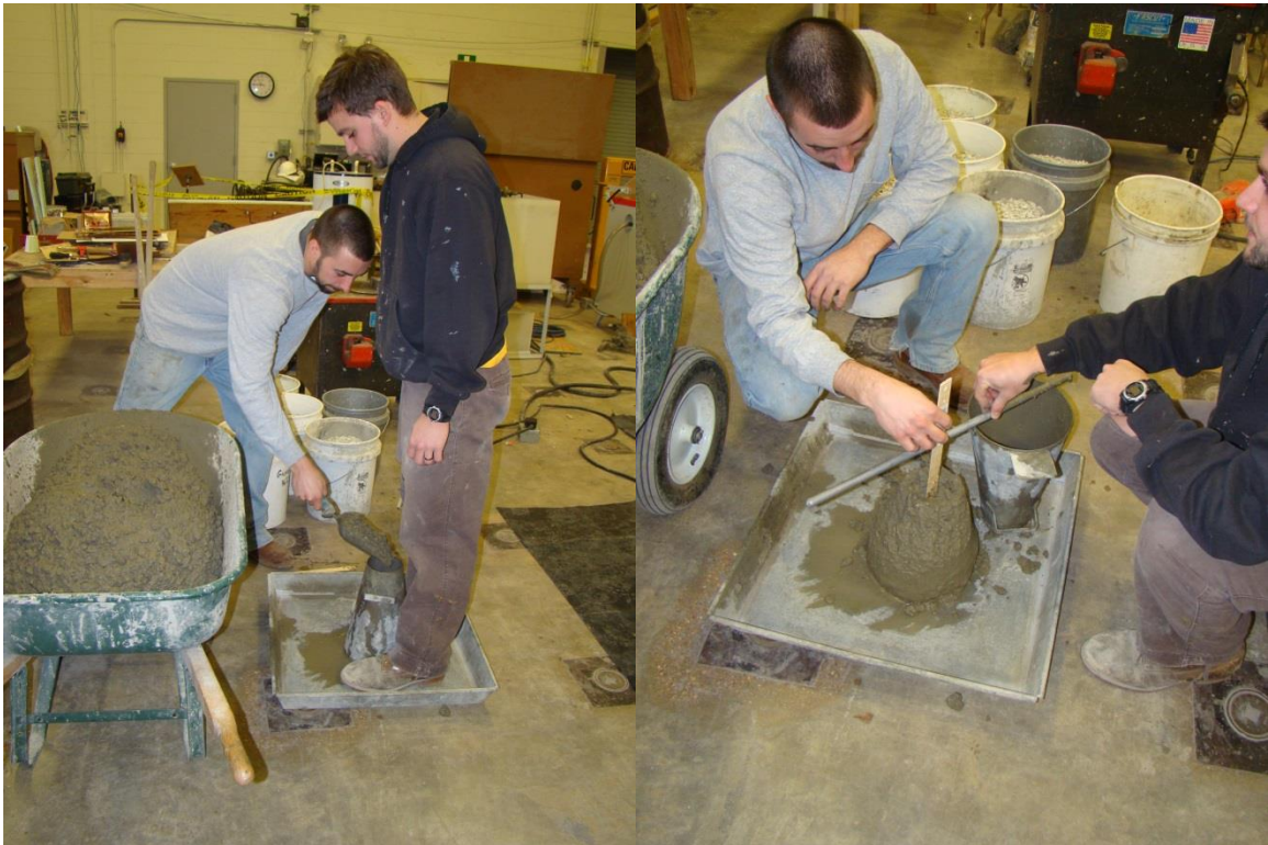
Figure 3.1 Slump test on concrete
