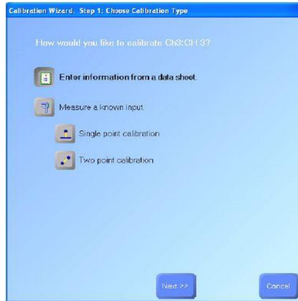
Figure 9.6 Calibration Wizard menu 1.
