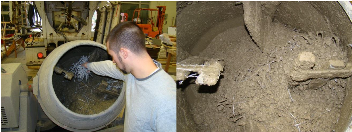
Figure 3.3 Mixing the LCFs by hand
