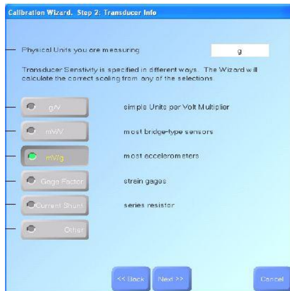
Figure 9.7 Calibration Wizard menu 2 units.
